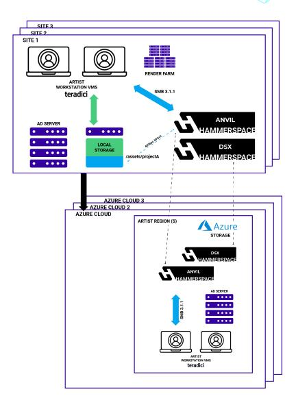
When Jellyfish leveraged Hammerspace to build a Global Data Environment, they deployed on-premises Anvil metadata servers, each with 4 DSX (data services) nodes. The nodes include high-speed NVMe SSDs connected to Hammerspace instances in multiple Azure regions. The Anvils work by replicating metadata between points in a bi-directional replication configuration. All sites are active, with all artists able to perform high-performance read/write on the same shared dataset.
